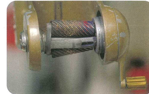
▲ If you take the cover off a pencil sharpener, you will find two screws that work together to grind away your dull pencil.
