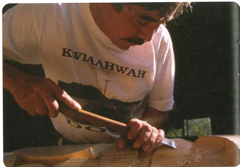
▲ The chisel that this carver is using is a wedge. The carver pushes the wedge to separate the wood.
